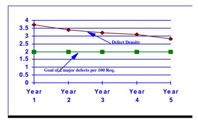
Figure 3: Defect Density Plotted Against Year
